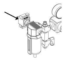
**3.** Attach grounding clamp assembly, P/N 17440-00, to the system mast clamp.
