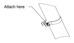
**4.** Securely attach Clamp, P/N 7749-00, to permanently grounded rod or pipe.
