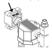
**8.** Open the air valve p/n 3165 on the solvent tank and adjust the solvent pressure to 90 PSI. (6 BAR) Open the ball valve p/n 18470-05 on the solvent tank. Next open ball valve p/n 23518-00 on the gun to verify that solvent will flow out of the front of the gun thru. the dispense tip, then close the valve.
