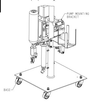
**b.** Lift to desired height, approximately 36" from the top of the base to the bottom of the pump mounting bracket. Use 3/4" wrench and tighten as tight as possible.
