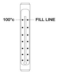
**16.** Fill the ISO pump lube bottle on top of the fluid section with DBP or material supplier's recommended lubricant.
