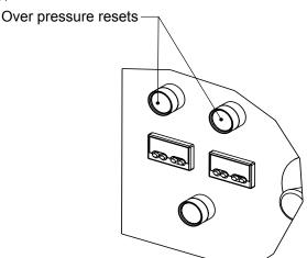
In an over pressure situation, the system will remain shut down until it is manually reset.
