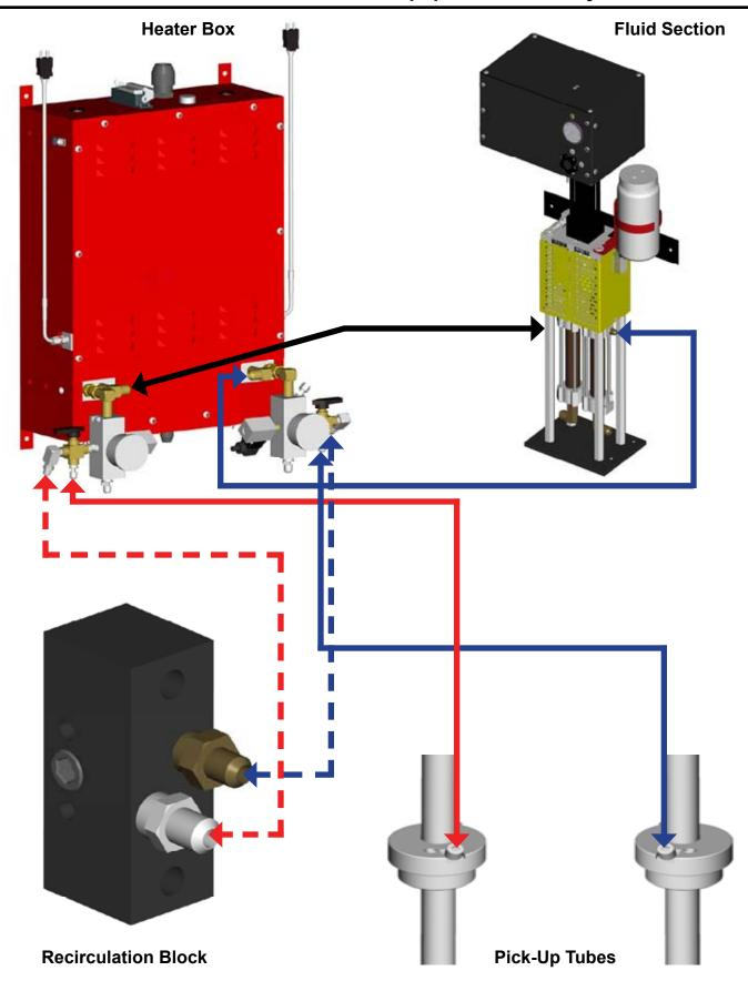
**Section 1 - Installation: Equipment Assembly**
