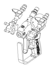
4. Place separate clean containers under each individual side block. Slowly open material valves (black arrow forward) on each side block to allow trapped air to escape the hose and material to flow into the containers until all air is purged from the material system.
